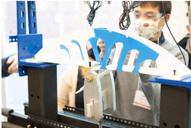
Figure B: Bridge loaded to failure
